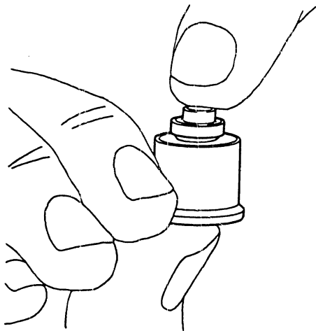
Fig. 42 Delivery valve inspection
